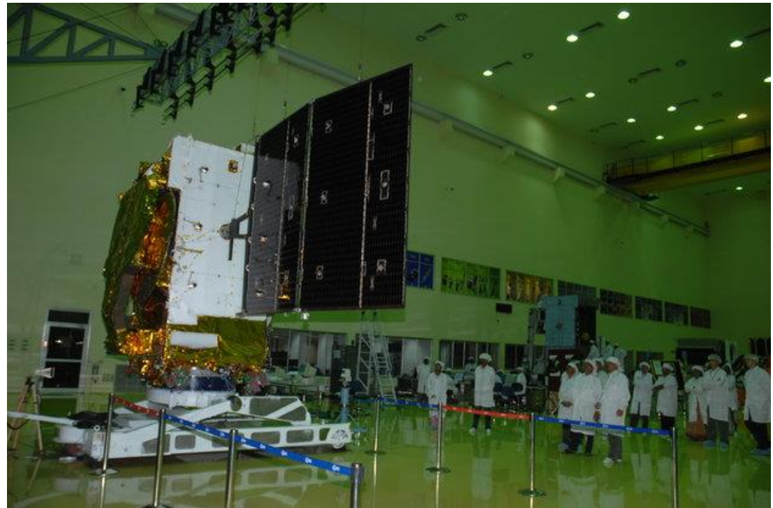
One of Hylas-1's twin solar arrays during deployment tests at ISRO Bangalore [photo: ISRO]
