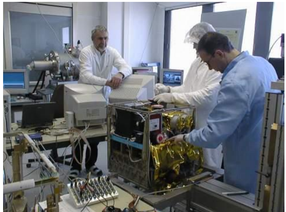
BIRD (P) FM at the fitting of the MLI [Photo: DLR]
