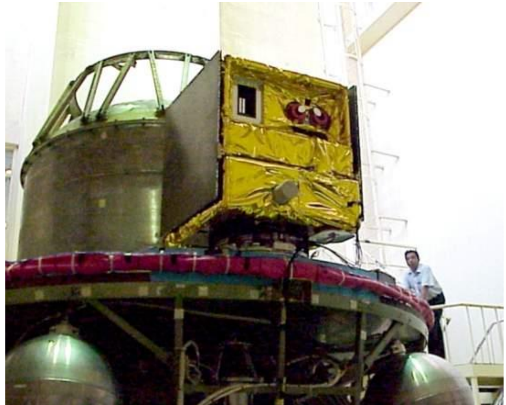
BIRD STM on PSLV-C3-upper stage for vibro tests [Photo: ISRO]
